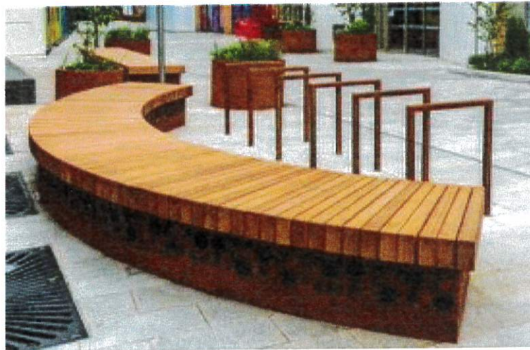
Coastal Path existing pathway with updated furniture, surfacing and furniture suited to match. Materials to be Corten etched steel, & timber. Existing mosaics to be retained.
